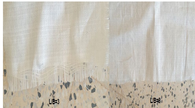
FIGURE 31: Damaged Ends of Shorter Woven Geotextile Compare to Longer One.
